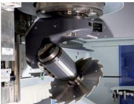
The powerful Drive 5CS 5-Axis spindle provides high dynamics and reduced contour interference
