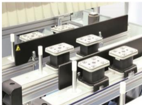
A rigid console table allows for flexible fixing of numerous vacuum and pneumatic clamping devices
