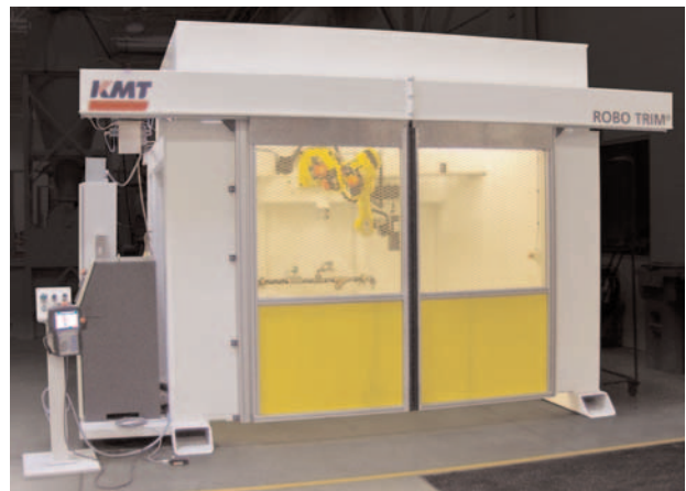
The RoboTrim FT-502 router trimming system, shown above, can trim parts up to 60" x 18" (or 1524 mm x 457.2 mm).
